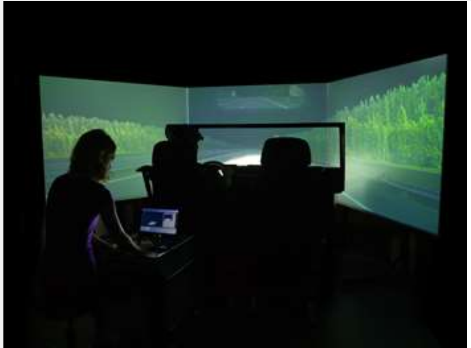
Figure: Simulated driving during a visual exploration experiment. The test subject wears a helmet with an integrated eye tracking camera to measure gaze direction.
